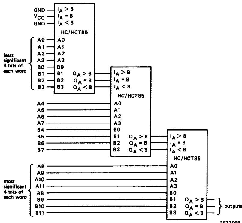
Fig.7 Series cascading; comparing 12-bit words.
