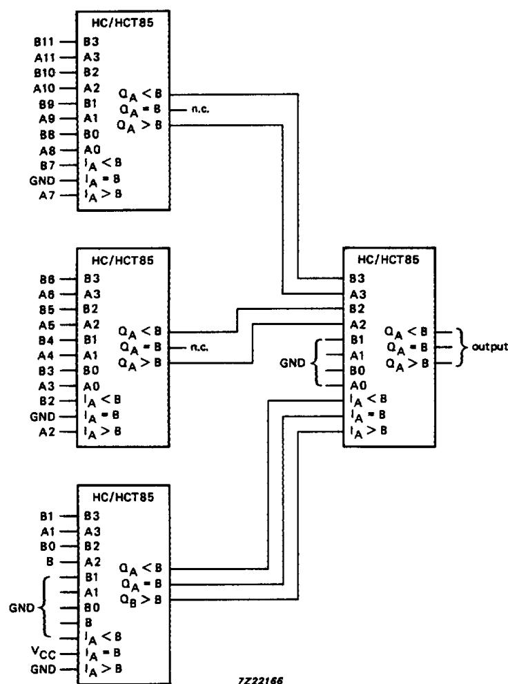
Fig.8 Parallel cascading; comparing 12-bit words.
