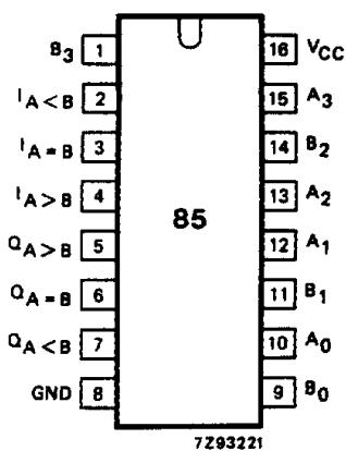
Fig.1 Pin configuration.
