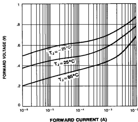
Figure 4. Forward Characteristics
