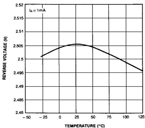
Figure 3. Temperature Drift
